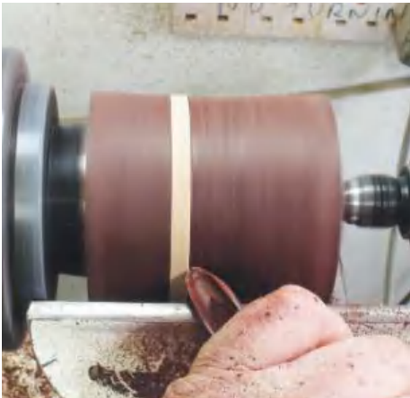
STEP 28. The piece can now be trued up using the spindle gouge; I am putting a slight concave shape across the joint to give the box a waisted appearance
